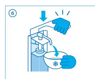
During this step, hold a collection container under the opening of the dispenser. Any product collected in the collection container can be disposed of in the sewerage system.
