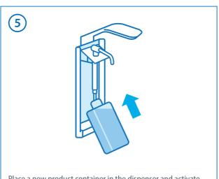
Place a new product container in the dispenser and activate the pump dispenser  $5\times$  to ensure an adequate dosing quantity.
