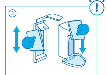
Clean the dispenser housing and the back of the dispenser as well as all external surfaces with a dampened (lint-free) disposable cloth. Disinfect the surfaces with a rapid disinfectant, ensuring that the exposure time is adhered to (DESCOSEPT PUR WIPES RTU, DESCOSEPT SENSITIVE WIPES).
