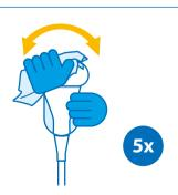
After the exposure time of CLEANISEPT WIPES FORTE / CLEANISEPT WIPES FORTE MAXI has been left on to take effect, dry the surface of the probe using a dry, lint-free disposable wipe.
