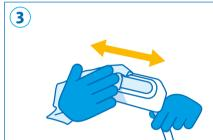
Dry probe with an additional disposable dry wipe.
