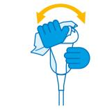
Enclose the wipe in your palm and rub it evenly across the surface of the probe five times using light pressure. Ensure that the entire surface is thoroughly moistened for optimal cleaning.
