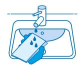
After removing the protective cover, wipe the probe with a commercially available, low-germ, lint-free disposable wipe that has been previously moistened with water.
