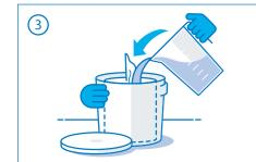
Slowly pour the disinfecting solution, in a spiral motion, onto the refill roll.
