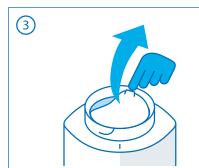
Pull the pressed-in membrane by the removal tab and remove it.
