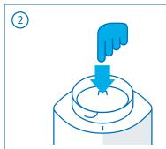
Press the membrane at the removal tab inwards.
